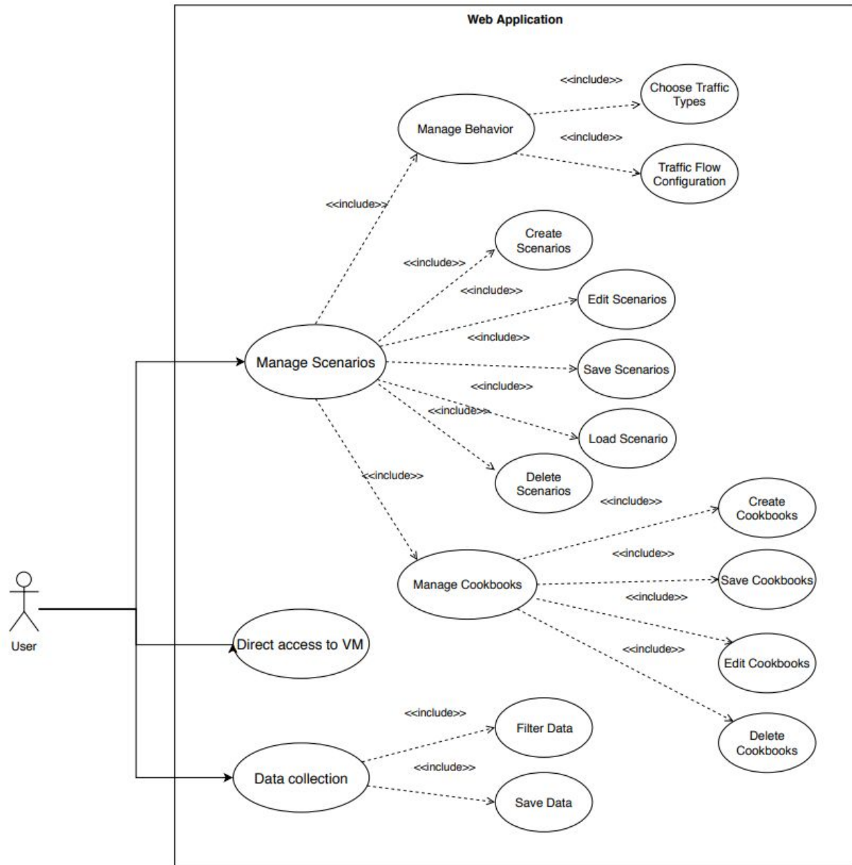
Figure 5: Use Case Diagram (Iteration 1) for Application
